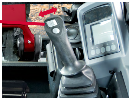
2 Proportional PTO control lever
