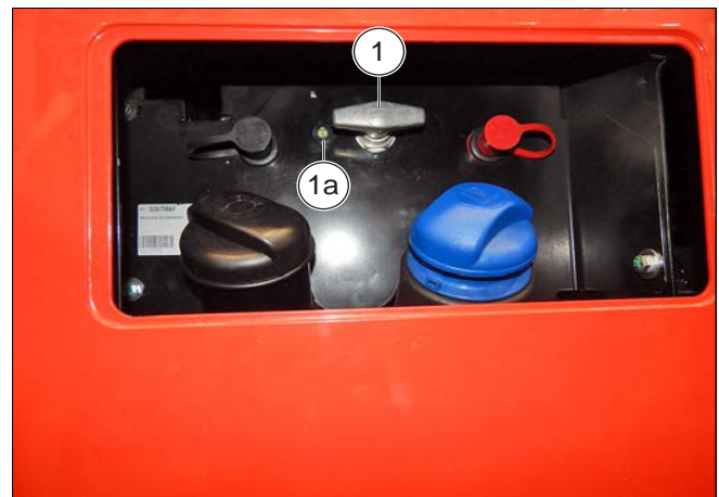
Figure 66: Battery disconnect switch
