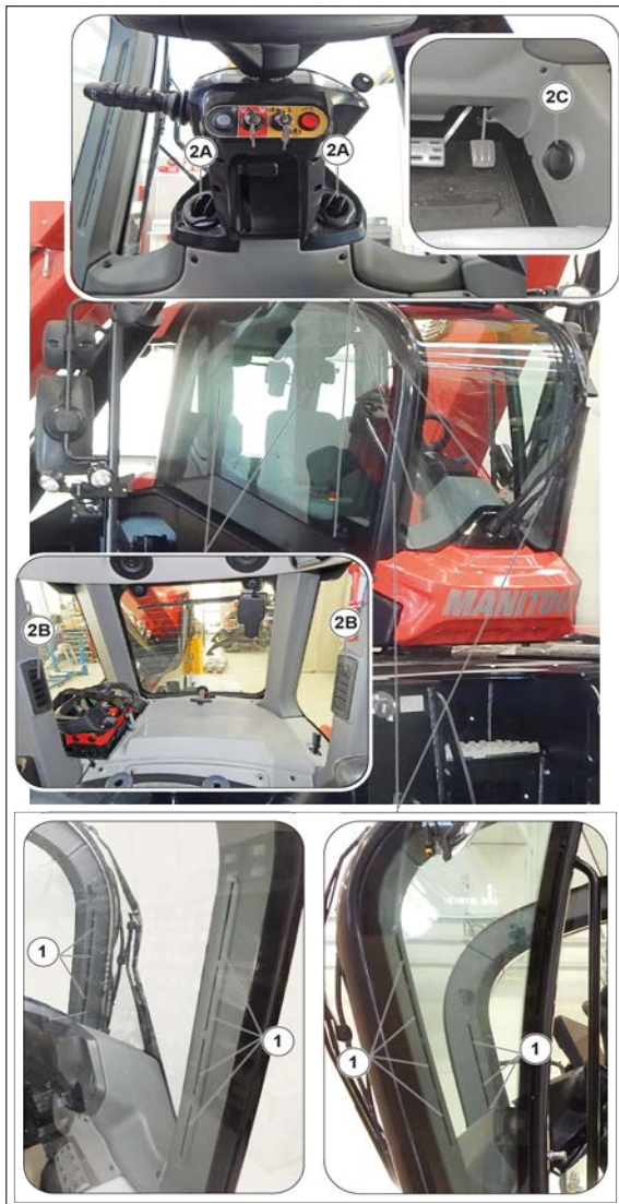
Figure 62: Demisting diffusers and heating air vents
