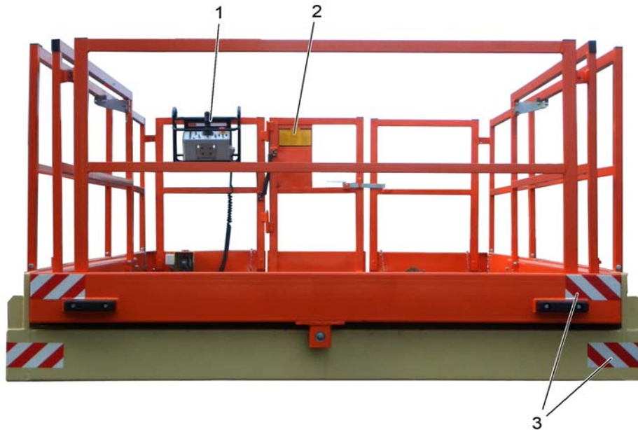
Decalls on the inside of the platform
