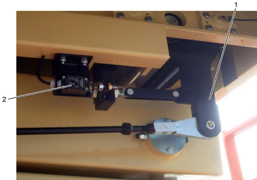
One of the overload safety device levers with switch
