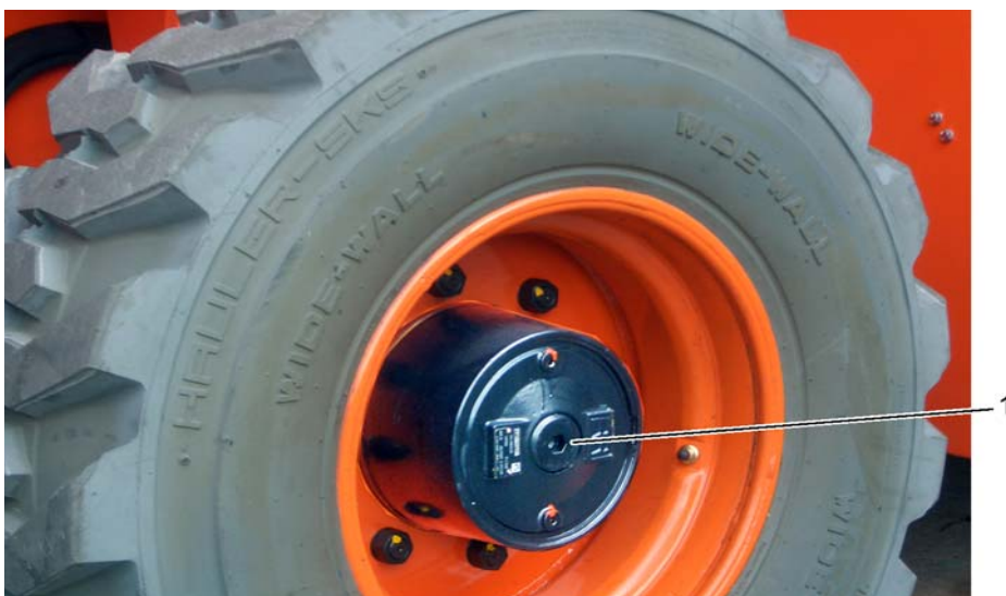
Releasing the multiple disc brakes
