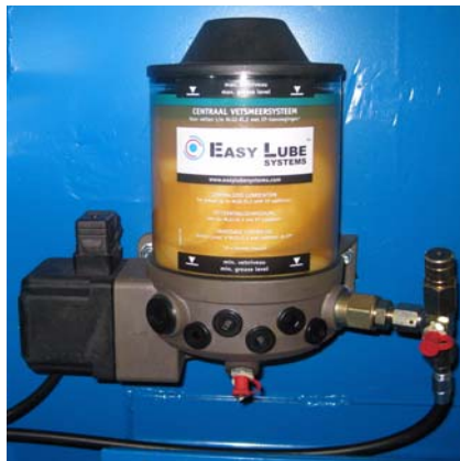
Easy Lube Systems™ grease reservoir
