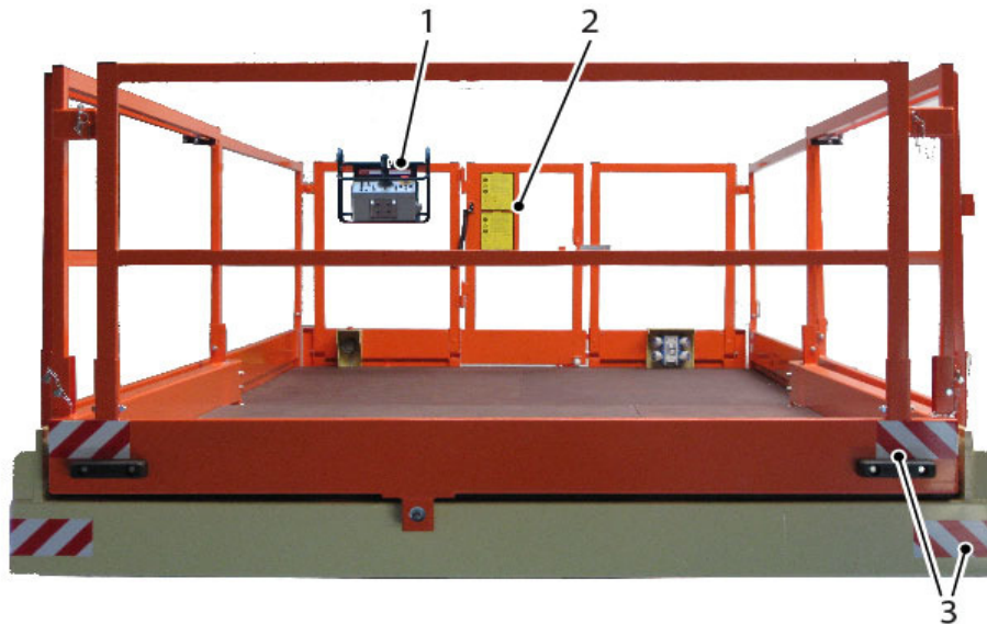
Decals on the inside of the platform
