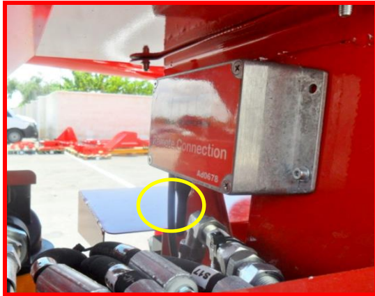
Picture 96: remote connection system.
