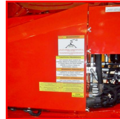
Picture 97: carter over the chassis box.
