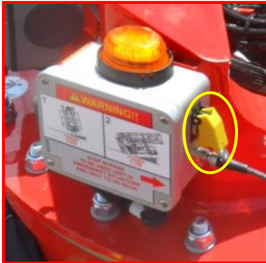
Picture 24: electric box for travel block bypass.
