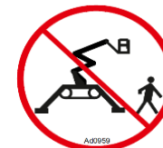
Picture 61: prohibition to stand in work area.
