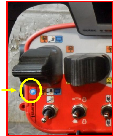
Picture 51: P button to bypass anti-collision system.
