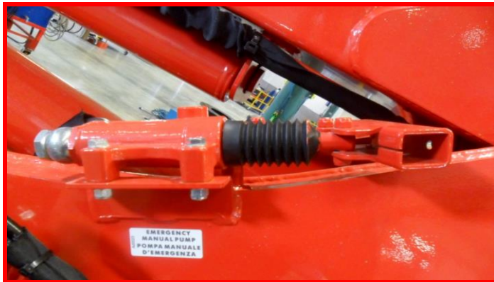
Picture 60: frame insert for manual pump.
