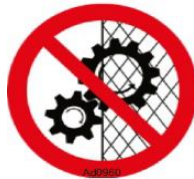
Picture 86: prohibition to remove safety devices.
