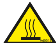
Picture 106: warning of burn risk.
