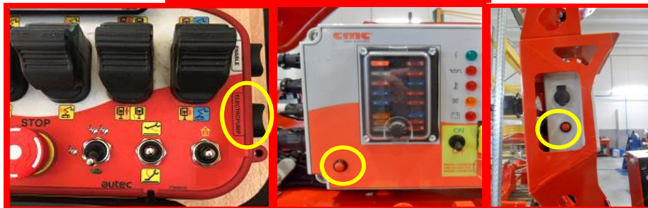
Picture 62: electropump (*optional) activation buttons.
