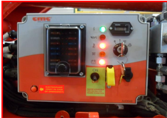
Picture 6: key position for ignition of endothermic engine from radio control or from basket console.
