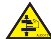
Picture 109: crushing and cutting hazard.
