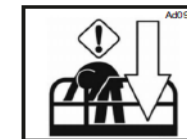
Picture 64: warning for basket operator fainting.
