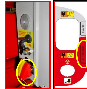
Picture 29: electropump activation buttons.
