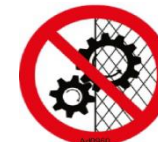
Picture 52: prohibition to remove safety devices.
