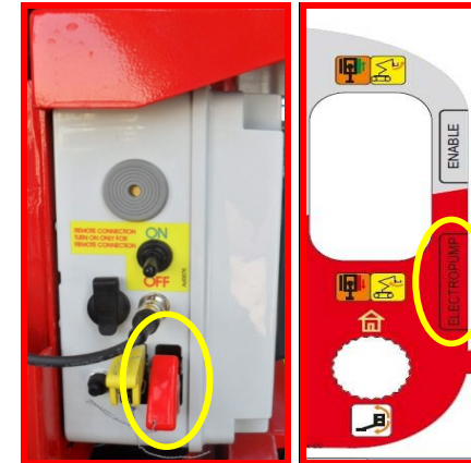
Picture 29: electropump activation buttons.
