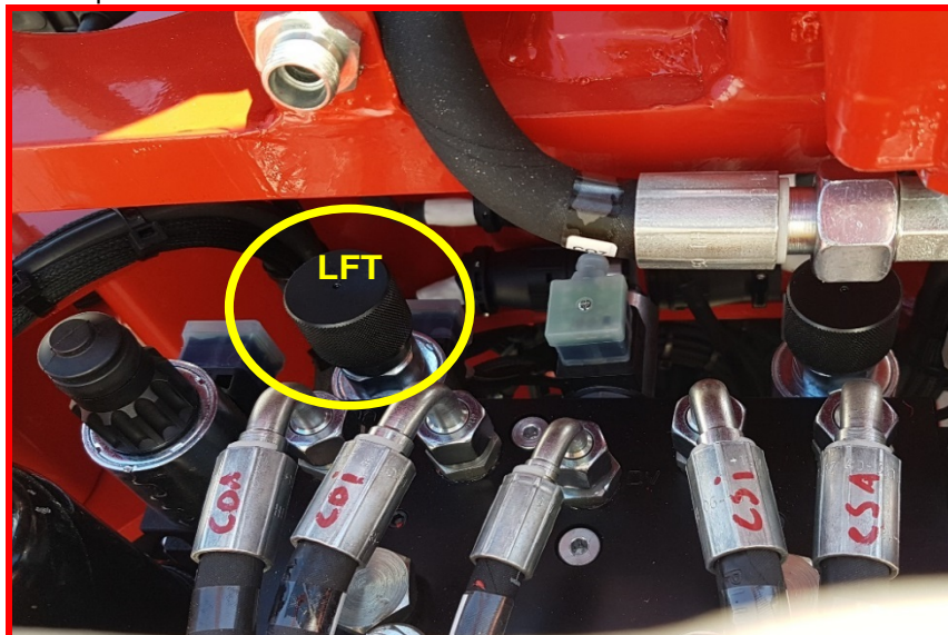
Picture 22: left filters bench tap.
