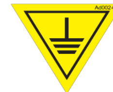
Picture 68: electric earthing.
