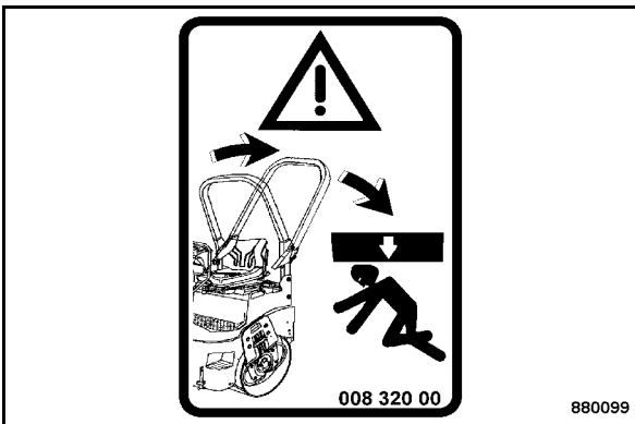
Fig. 10 Warning sticker - Foldable ROPS 1
